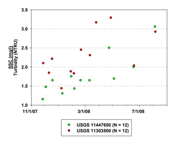
Figure 7. Ratios of suspended sediment concentration (SSC, mg/l) to turbidity (NTRU) in data collected from USGS stations from October 2007 to August 2008. Source of data: http://waterdata.usgs.gov/usa/nwis/sw.
