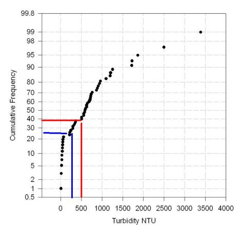
Figure 5. Cumulative percentile plot of Caltrans turbidity data, based on 49 data points collected during water year 1999/2000 and 2001/2002 (no data were collected during water year 2000/2001; Caltrans 2002). The data in the Caltrans (2002) dataset would exceed the proposed NEL of 500 NTU 60% of the time and would exceed the proposed NAL of 250 NTU 75% of the time.
